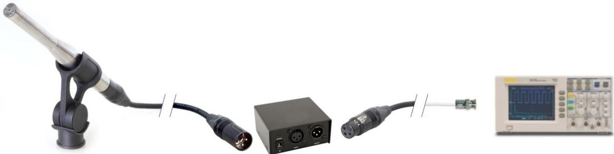
*Phantom Powered Microphone System*
