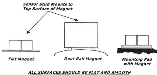
**Figure 6.** Magnet Mounting Types
