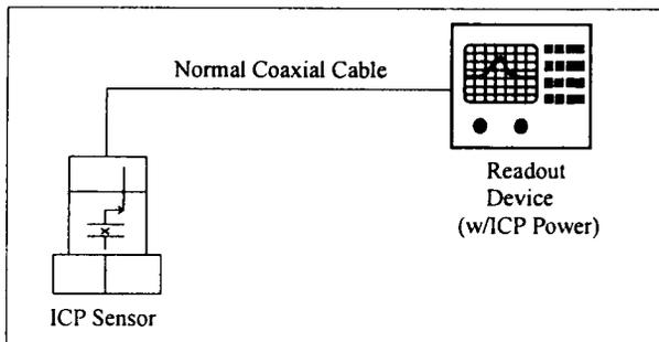
Figure 17. ICP<sup>®</sup> Sensor System Connector
