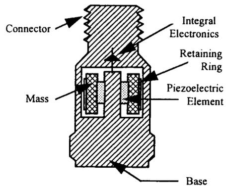
Figure 1. Typical ICP<sup>®</sup> Industrial Shear Mode Accelerometer
