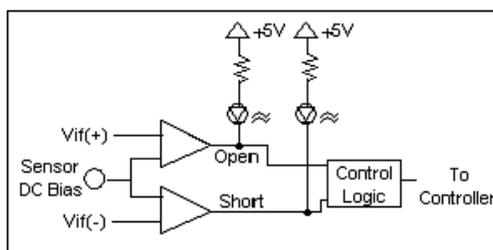
Figure 3 Input Fault Window Comparator with LED Indicator
