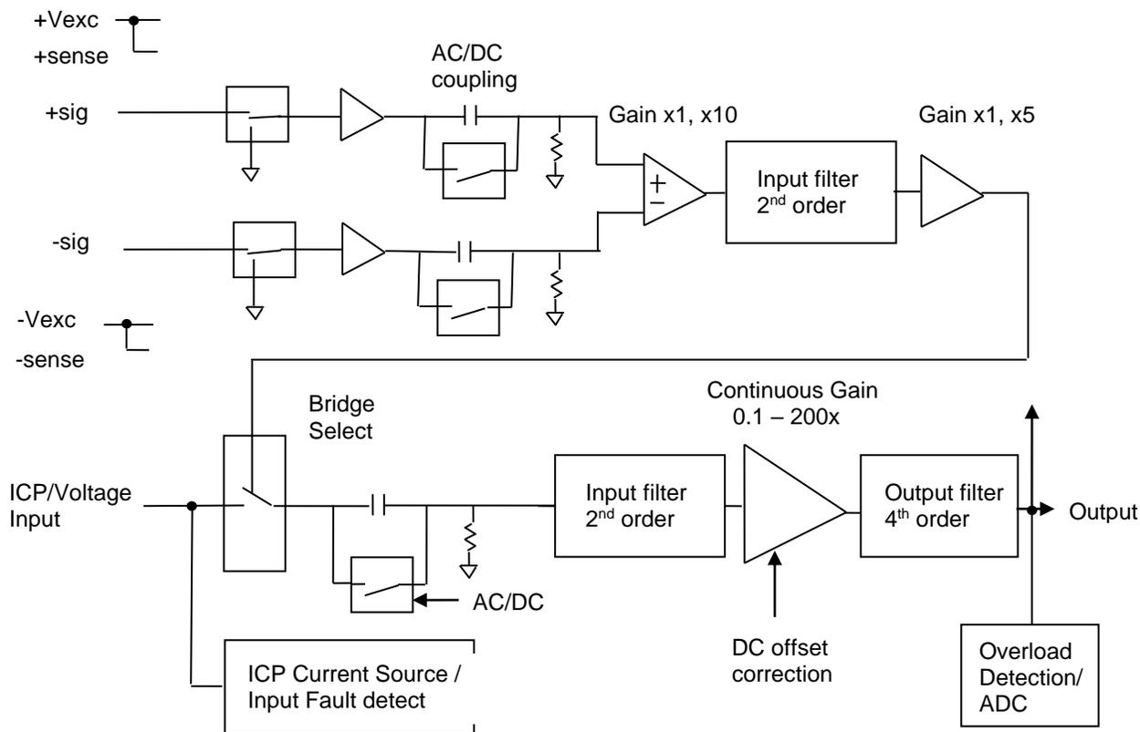
Figure 1 Typical Block Diagram of Model 482C27
