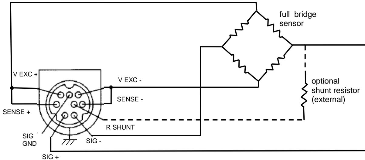
**Figure 7 Alternate Connections for Differential Voltage/Full Bridge Type Sensors
