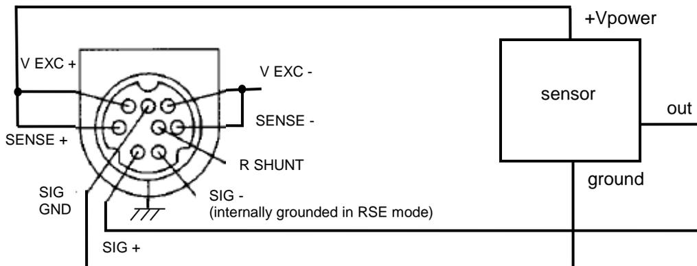
**Figure 10 Recommended Connections for 3 Wire Type Sensor
