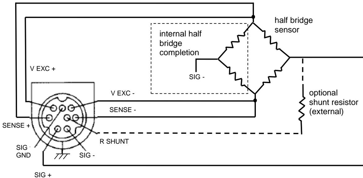
**Figure 8 Recommended Connections for Half Bridge Type Sensors
