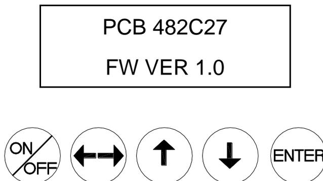
▼ This button is used to scroll DOWN through the options in the menu. In the submenu, this button can be used to change the channel and increments.
