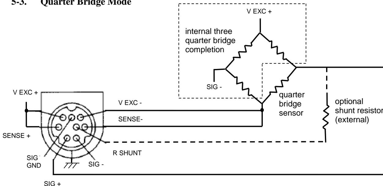
**Figure 9 Recommended Connections for Quarter Bridge Type Sensors
