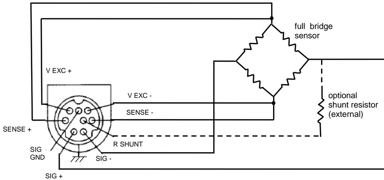
**Figure 6 Differential Voltage/Full Bridge Type Sensor Connections**
