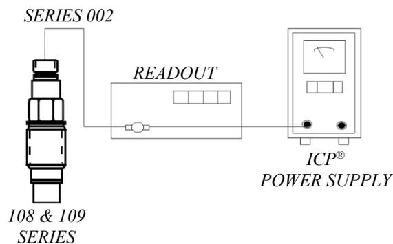
With this arrangement, the readout is direct-coupled to the sensor and the output signal will be added to the DC bias voltage (11 VDC nominal).
