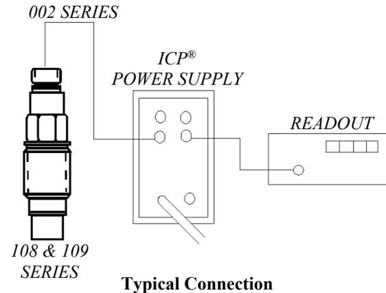
The figure above shows the 108 & 109 Series connected to a PCB Model 484B06 power unit. The 484B06 is a power unit that can be AC or DC-coupled.
